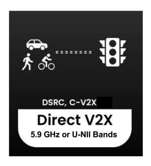
Direct V2X provides low-latency communication between entities for safety critical applications. Requires special hardware in vehicles.
